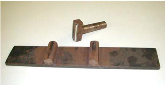
twenty inches long. It fits across the big plate you saw bolted to my flypress and I clamp it down with a couple of small welding clamps. Another bread-loaf bar is welded to a stem for my top tool. These bread-loaf bars are all just mild steel.
