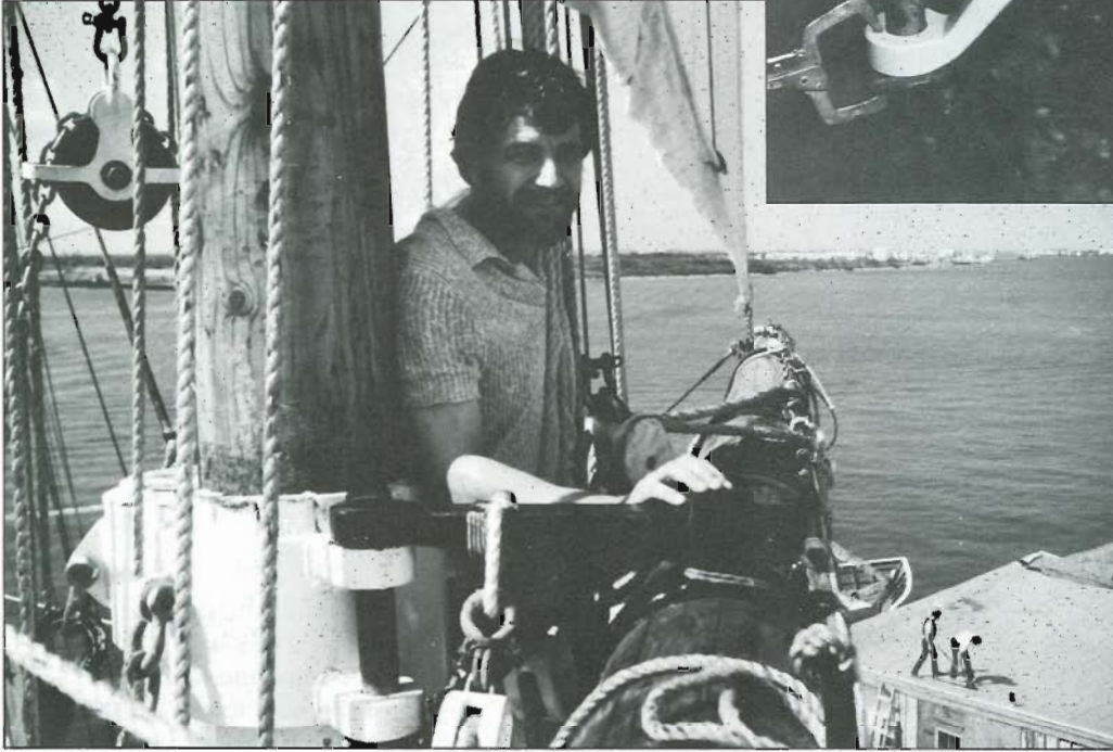
Lower topsail yard crane installed.
